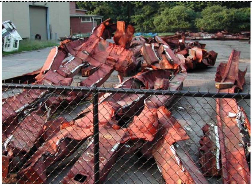
Figure 160. WTC beams with spandrel plates wilted like tissue. (9/05): NCSTAR1-3c-P187_carpet_c.jpg
